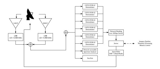
Figure 5: Block diagram of the six channel HSD2-capable ground station.
