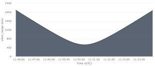
Figure 9: The slant range to the satellite as a function of the UTC time during the pass. The distance between the ground station and the satellite changes from over 2000 km at 5 deg. elevation to 530 km at 71 deg. elevation.
