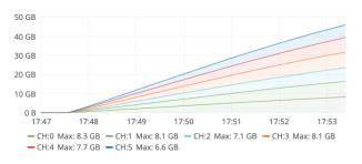
Figure 7: Six channel HS2 system downloaded 46 GB of data December 12, 2018.
