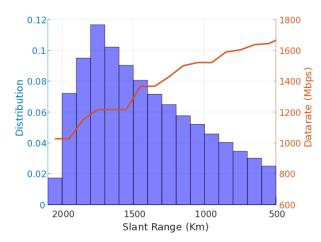
Figure 15: The histogram of slant ranges from a Dove satellite in a 500 km SSO orbit is shown in blue and the predicted data rate as a function of slant range from the HSD2 channel simulator is shown in red.
