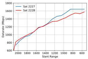
Figure 16: Data rate measured at the Keflavik ground station from the F4A satellites 2227 (blue) and 222B (red) over a three week period from May 20 to June 11, 2019.
