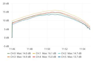
Figure 10: The demodulator recorded signal to noise ratio (SNR) is shown for the six channels at the ground station.
