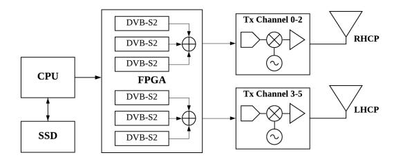
Figure 2: Block diagram of the six channel HSD2 satellite transmitter.
