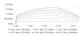
Figure 12: The data rate recorded by the demodulator shows max data rates between 248 Mbps to 311 Mbps for the six channels.
