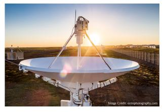
Figure 3: 4.5 m diameter S/X dish in Keflavik, Iceland.
