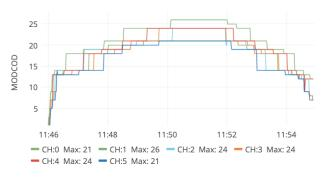
Figure 11: MODCOD is adaptively incremented or decremented based on link availability by the ACM algorithm on an individual channel basis. The modulation changes from QPSK at the start of the pass to 16/32APSK at the middle of the pass for various channels.
