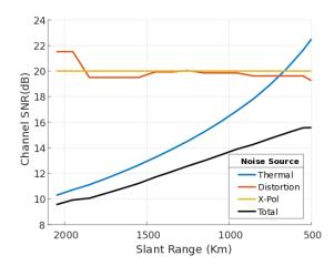
Figure 14: Black curve shows the total simulated SNR at different slant ranges. Contributions from various sources are shown with thermal noise in blue, signal distortion in red and cross polarization in yellow.
